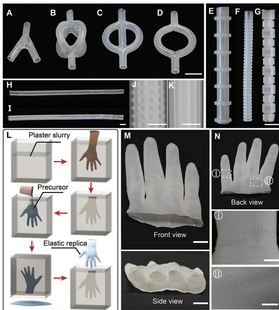
Figure 3. Soft shells with complex geometries and elaborate structures. A–D) Soft shells with inner connection structures, including a three-branched tube, a spherical-branched tube, a “ \Phi ”-shaped branch tube, and a circular-shaped tube. Scale bar, 1 cm. E–G) Soft shells with uniformly distributed topological geometries, including circular edges, corrugated geometries, and segmented gear structures. Scale bar, 1 cm. H–K) Soft shells with microstructures. H) Shows a shell with microstructures of papillae, and J) Zooms in the microstructures. I) Shows a shell with microgrooves, and K) Zooms in the microstructures. The scale bars are 2 mm in (H, I) and 1 mm in (J, K). L) Fabrication process of the soft replica of a human hand. M) The front and side views of the soft shell of a human hand replica. Scale bars, 2 cm. N) The feature parts of the replica. Scale bars, 5 mm.
